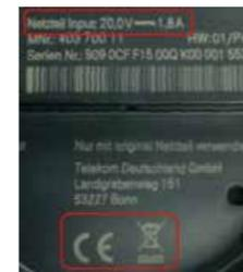
As shown in the figure above, Netzteil Input is the power input required for this product. CE is the EU safety requirement compliance mark. The crossed out trash can symbol reminds the user not to discard the product directly into the trash can but to follow the recycle directive instead.
